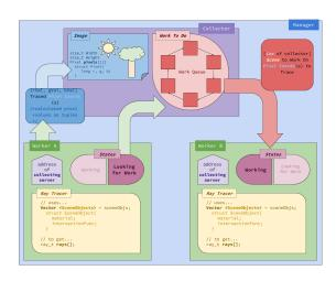
This diagram shows two Workers and one Collector. The Collector produces an image with an arbitrary width and height. The Collector can be in one of two states: assigning work, and outputting image. When the Collector is assigning work, it waits for messages from Workers, then allocates work to each Worker that asks. The Collector selects work based on the current front of a circular queue. Once work is complete (read: returned by a Worker), it is removed from the queue.
